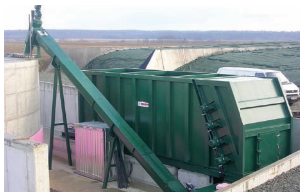
Photo 7: Silage dosing unit (back) with spiral elevator (front). The silage clamps can be seen in the back.
