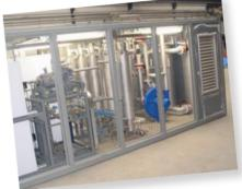
Since gas cleaning and  $CO_2$  extraction are combined, it is not necessary to remove the sulphur beforehand. Methane losses are low: max. 0.5%. GTS supplies standard systems that can cope with 50–2500 Nm<sup>3</sup> biogas per hour.
