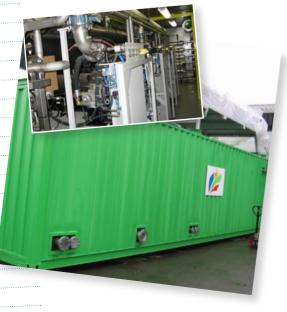
Van der Wiel Stortgas This company offers a wide range of solutions and services regarding environmental techniques. In order to upgrade biogas to natural-gas quality, Van der Wiel supplies equipment that can cope with an input of 200–3000 Nm<sup>3</sup> per hour.
