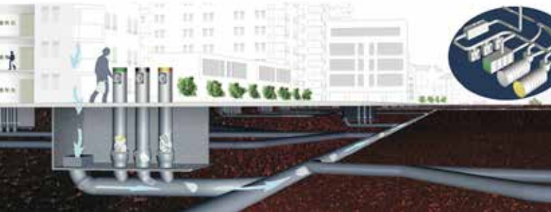
Figure 23: Picture of a stationary vacuum system (Source: Envac)
