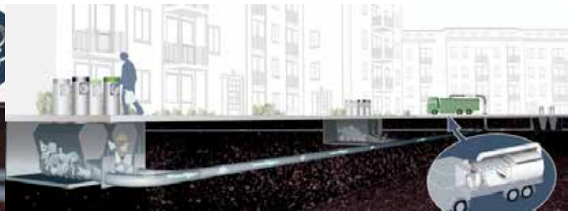
Figure 24: Picture of a mobile vacuum system (Source: Envac)
