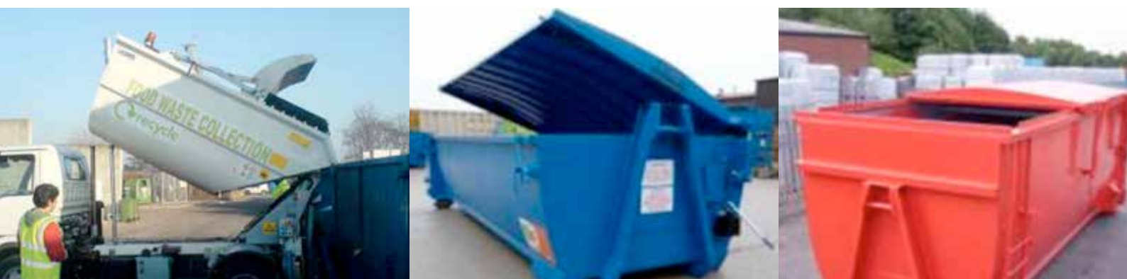
Figure 26: Bulking of organic waste in containers. Collection vehicle tipping (left) into a waste container (middle and right).
