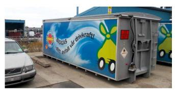
**Figure 4:** Container used for transportation of compressed biomethane in Sweden. The container is filled with high pressure gas cylinders.
